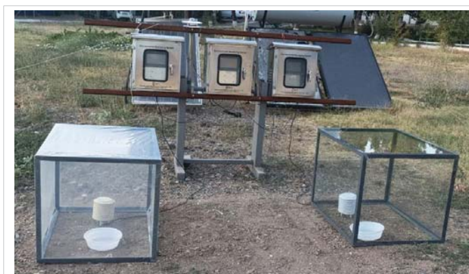
Figure 2: General view of the boxes with transparent walls during the experiments on the study of heat losses.
